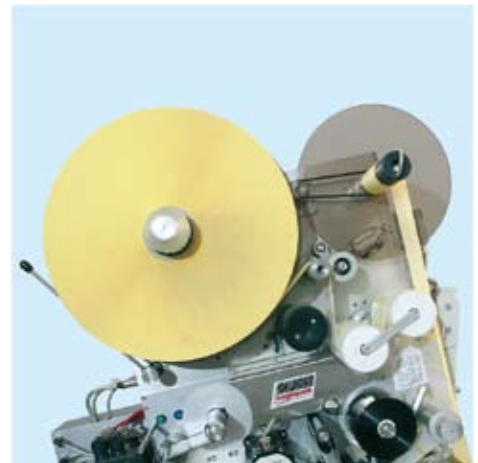
Jumbo roll unwinders with 1200 m stock
